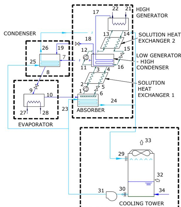
Figure 2. Control Volumes for the Thermoeconomic Functional Analysis – Double-Effect System.
