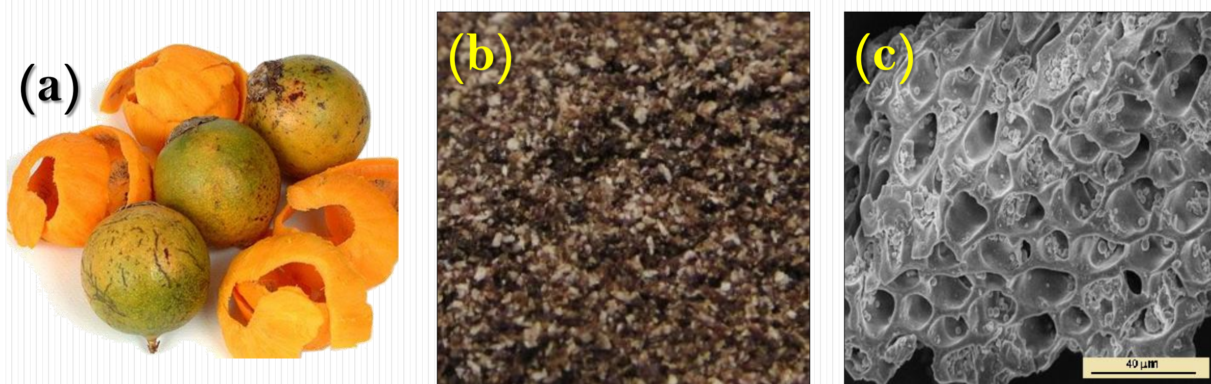
Figure 2. (a) Tucumã's fruits, (b) tucumã seed in natura after preparation and (c) SEM image of tucumã seed.
