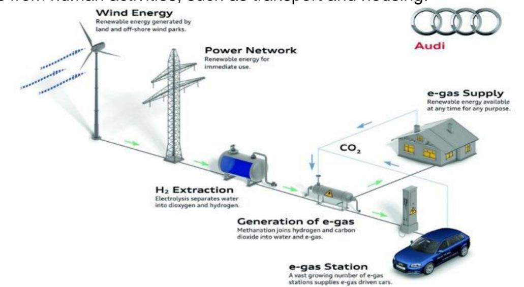
This paper considers the catalytic hydrogenation of the captured CO2 (also known as the Sabatier reaction) to synthetize methane, the Sabatier reaction states that it is necessary 5.5 kg of CO2 for each kg of H2 in order to obtain the stoichiometric composition of methane [2], or in other words, in order to produce each kg of CH4 it is necessary 0.5 kg of H2 and 2.75 kg of CO2.
