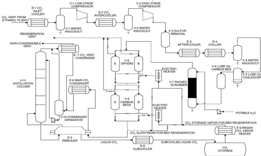
Figure 1. Schematic of the CO2 capture plant considered in this work Source: [2] (Illinois State Geological Survey, 2006)
